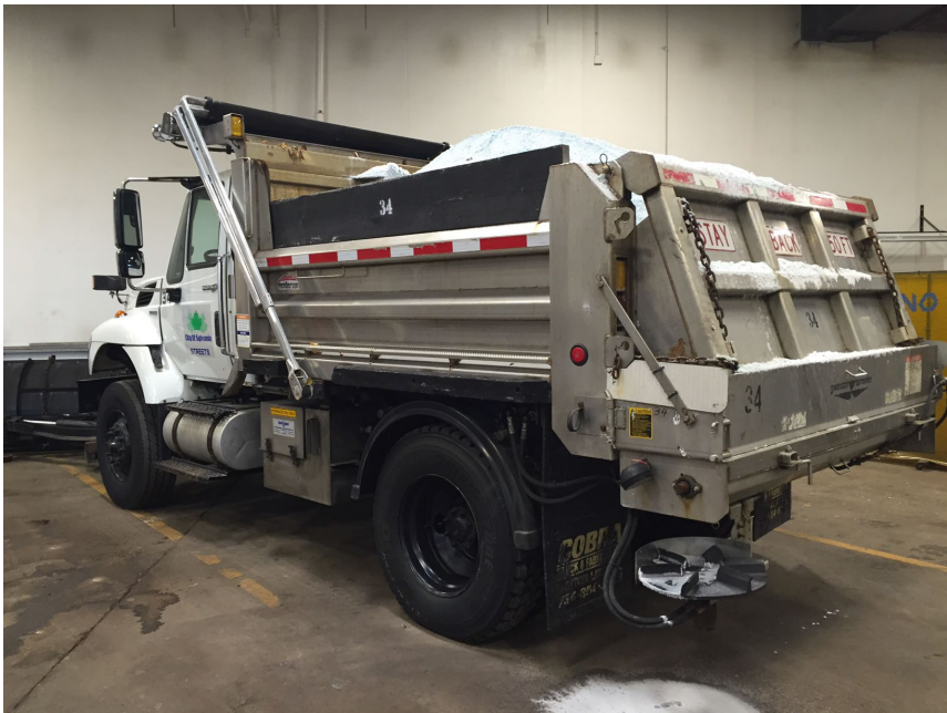
City truck equipped with salt spreader
