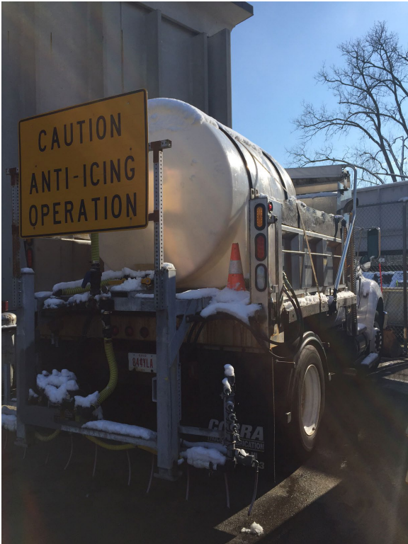
City truck equipped with brine tank and spreader
