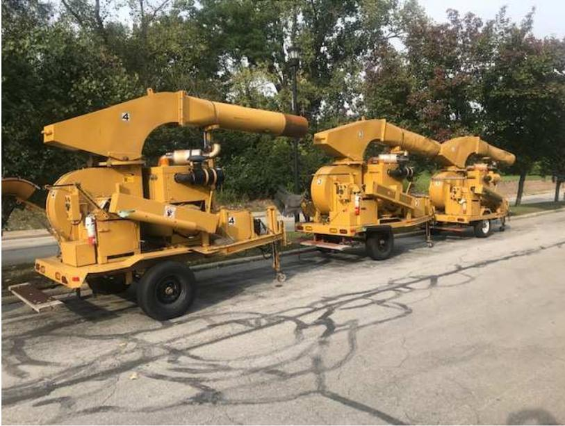
Three diesel powered leaf loader vacuum units.
