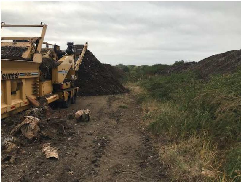
Leaves and green yard waste being ground by horizontal grinder and stacked into wind rows.
