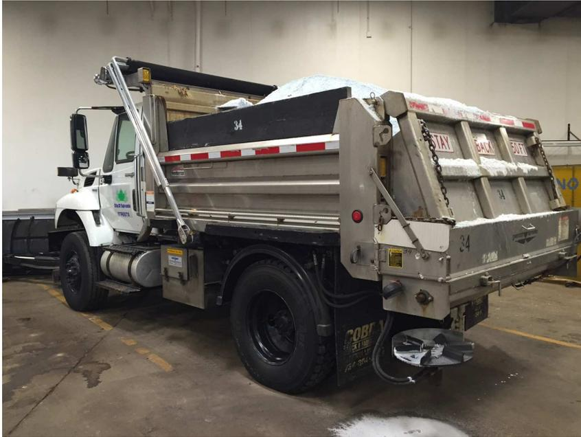
City truck equipped with salt spreader
