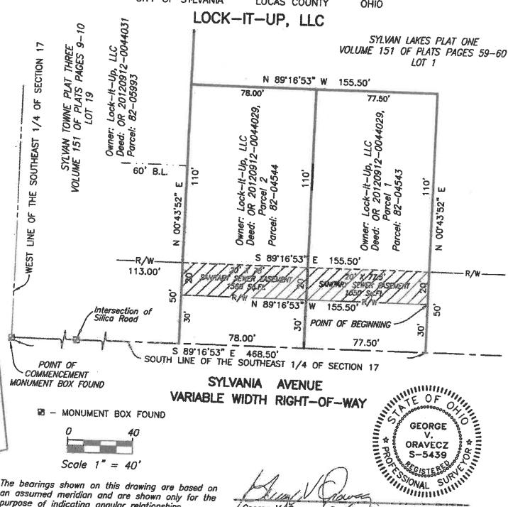
The bearings shown on this drawing are based on an assumed meridian and are shown only for the purpose of indicating angular relationships.
